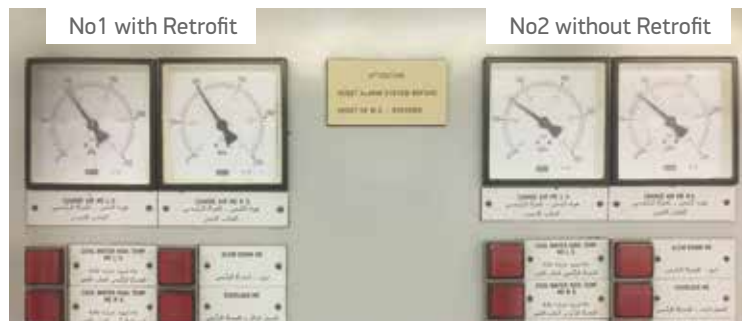
Pressure Indicators of a Passenger vessel with 2 M/E Pielstick 12PC2-5V. Monitoring both engines in the same load:
